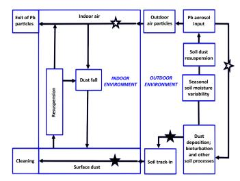
**Fig. 2.** Environmental signaling within the context of individual properties of the city (after refs. 38, 56). Key components are inputs of air Pb, SPb deposition, and Pb particle resuspension that serve as environmental signals in children's inhalation (open stars) and hand-to-mouth (closed stars) routes or pathways of exposure.
